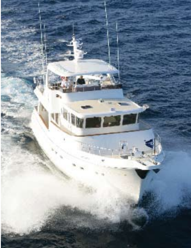
Barely visible below the surface in this picture taken off the bow, Southern Pearl has the optional bulbous bow, which combined with KeyPower fin stabilizers, improves ride in heavy seas. Above right, generous cockpit seating will keep the captain in the heart of the gathering. Below right, the gentle sweep of the stern can be seen in the curved bench seat with cockpit table.
